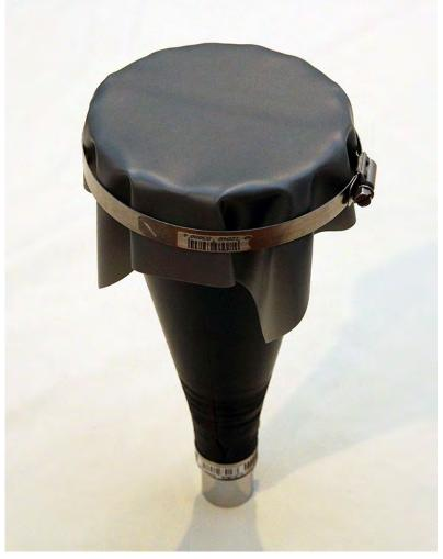
...and, using the screwdriver, tighten it around the funnel to securely hold the screen; as the clamp begins to get purchase on the funnel and screen, gently pull down all around the loose edge of the material so that the screen ends up flat and taut over the funnel's wide opening. This is an iterative process; you'll need to pull down on the material after each turn of the screw to keep it taut.
