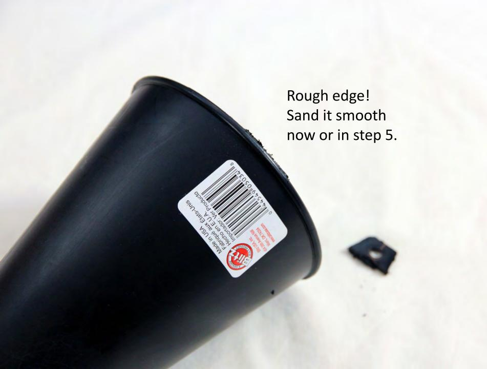
**Step 3.** Using the hacksaw, cut about 7 inches off the narrow end of the funnel so that what's left measures about 10 inches long (use the ruler).
