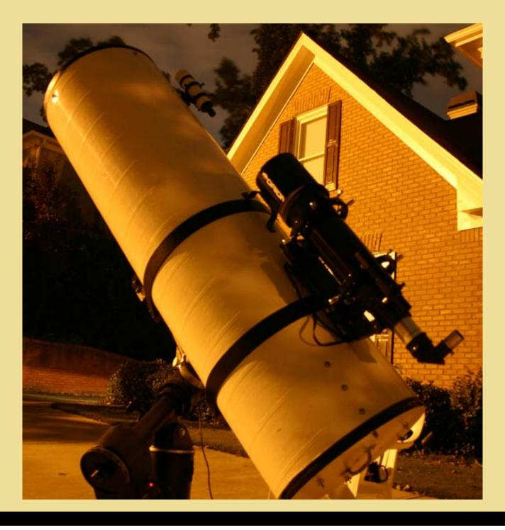
Larry gave us an update on the latest testing and modifications to the club's Starfinder 16 EQ. Here the new dovetail accessory plate is shown with an Orion 5" refractor attached as a finder scope.
