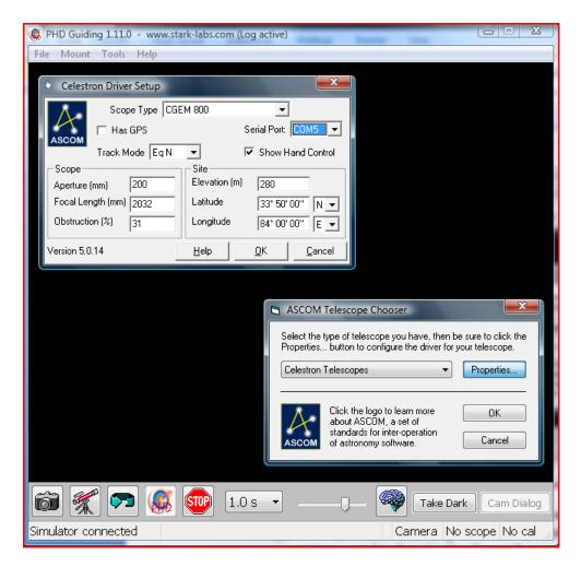
Select your scope from the ASCOM Telescope Chooser dialog that appears (lower right above). Then click Properties and the driver setup dialog for your scope will appear (upper right above). Configure the mount type, serial port connection, hemisphere, and check hand control if you want to move the scope around from inside PHD. Correctly setting the COM port is essential to connecting to the telescope. Verify the status bar confirms successful connection to the mount.
