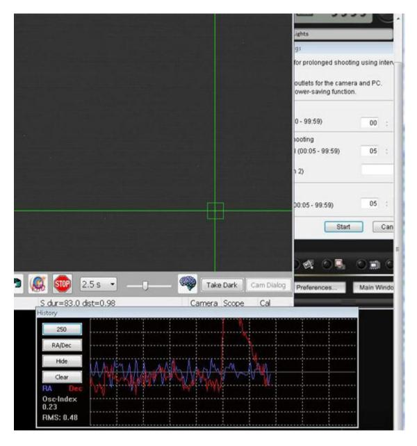
The guide graph will plot two horizontal lines showing the guide star drift in RA and Dec from the position PHD is trying to hold the guide star at. A big Dec excursion is shown above, usually caused by a problem in or at the mount. As PHD issues corrections to the mount, hopefully you will see the horizontal lines return to the solid line at the center of the graph. Each dotted horizontal line represents a one pixel deviation of the star on the guide camera. Whether this is going to harm your
