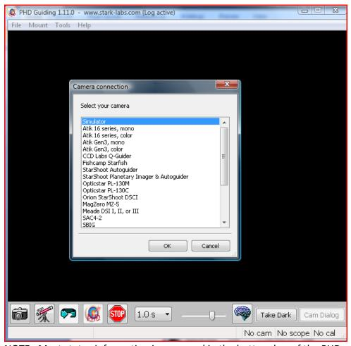
NOTE: Most status information is conveyed in the bottom bar of the PHD screen below the icons at the bottom of the screen. Not very eye catching and in my opinion, too easy to miss. In the screen above, the status displays No cam, No scope, No cal which means PHD isn't connected or calibrated.
